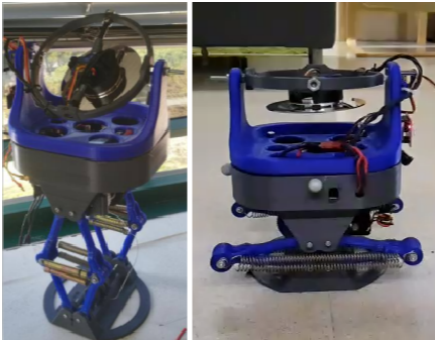
Figure 1: The Moonhopper. Extended and compressed configuration
